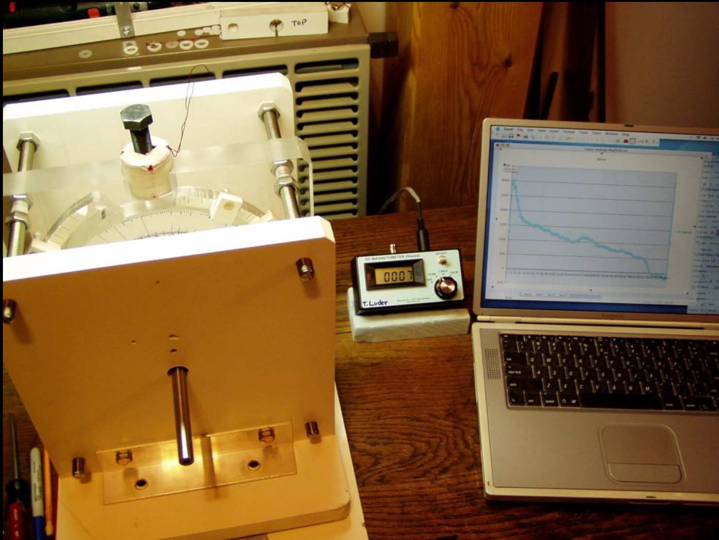
Overall setup used to measure initial gauss field. Readings were typed directly into the computer. Gauss meter is in the center.
