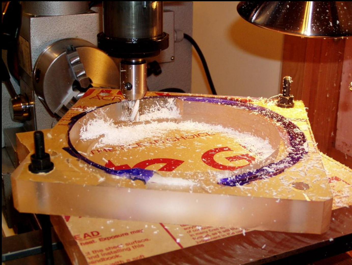
Machining spiral in Plexiglas stator version 2.0.
